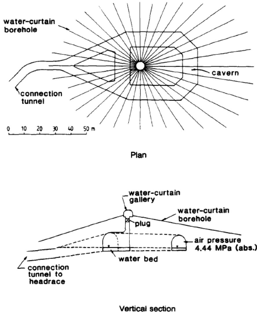
Figure 5-3: Water curtain of an air pressure cavern constructed for a hydro power project [14]
