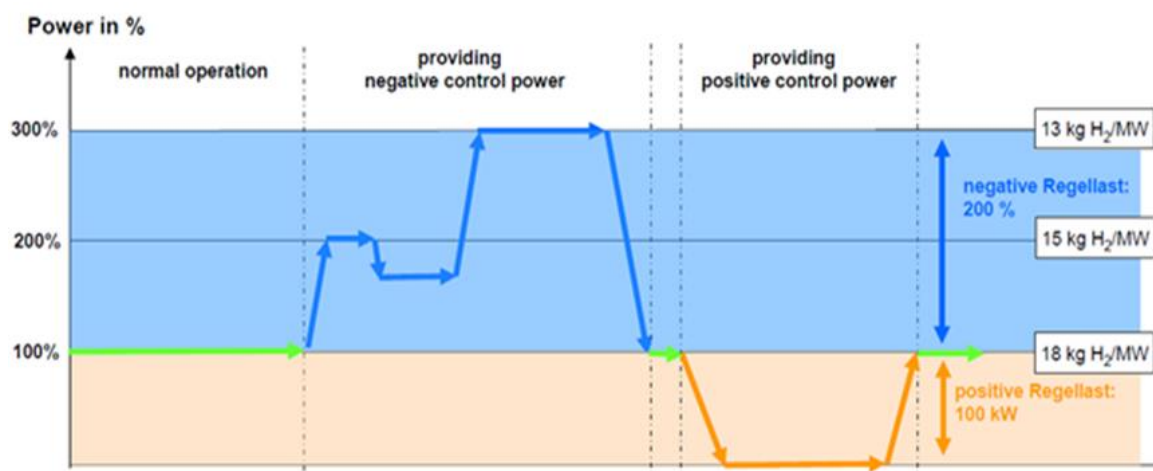
Figure 4: Example for capabilities of PEM electrolyzers for hydrogen production in DSM systems (Source: [Waidhas 2011])
