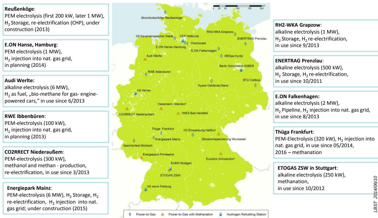
Figure 10: Power-to-Gas – demo projects in Germany 2013 (Source: LBST)
