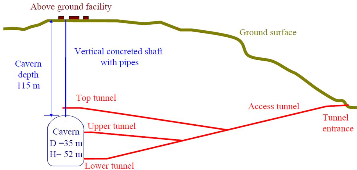
Figure 5-8: LRC Skallen schematic of cavern setup (bottom) [41]
