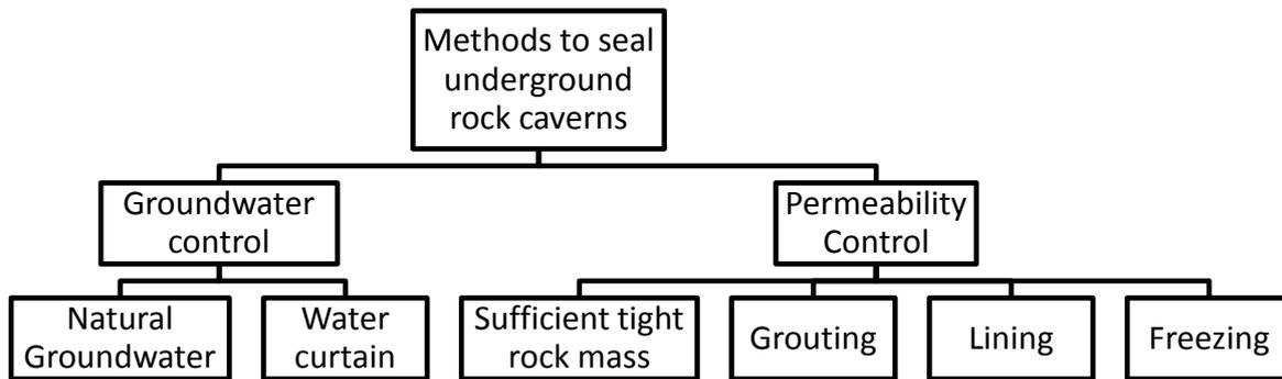
Figure 5-1: Methods to limit or eliminate gas leakage from a pressurised underground storage, after [14]
