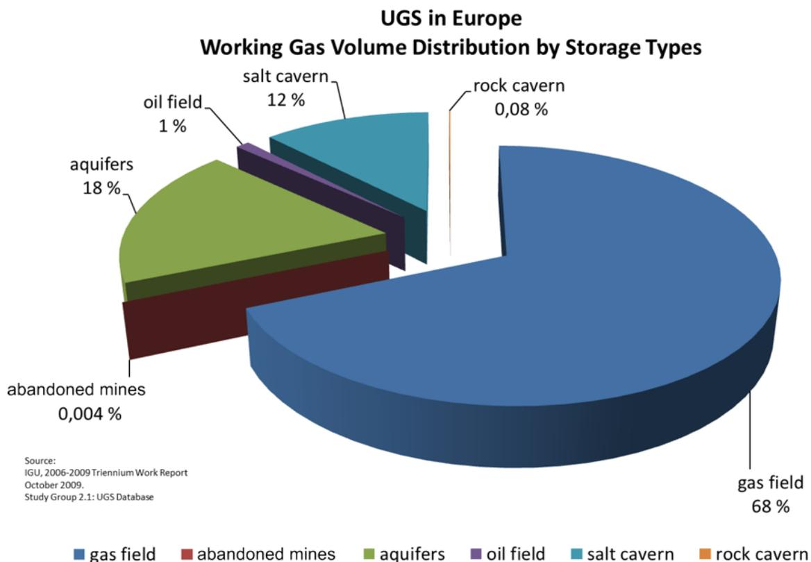
Figure 1-1: Distribution of natural storage options (basis: working gas volume) [30]
