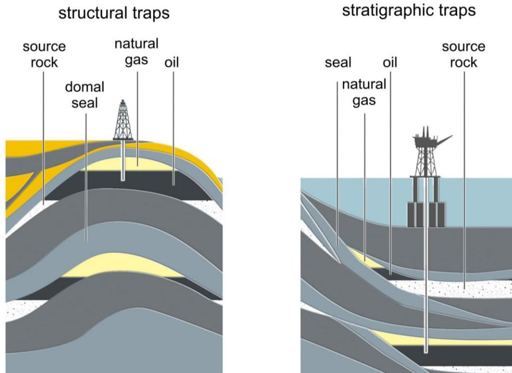
Figure 4-2: Classification of traps, [32] modified by KBB
