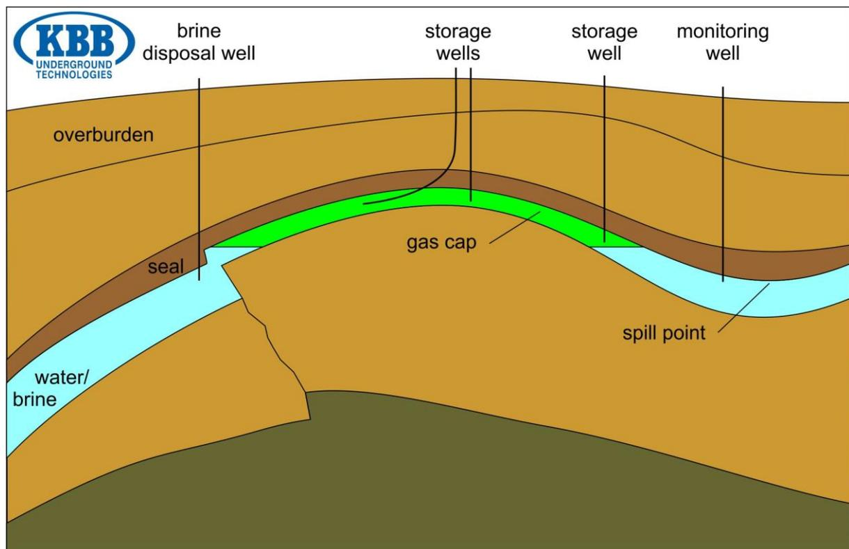
Figure 3-1: Sketch of gas storage in an aquifer.
