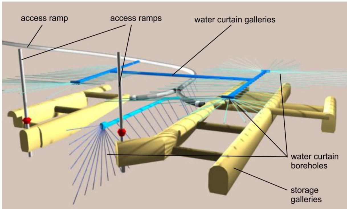
Figure 5-2: Storage galleries and water curtain of LPG storage, after [36] modified by KBB
