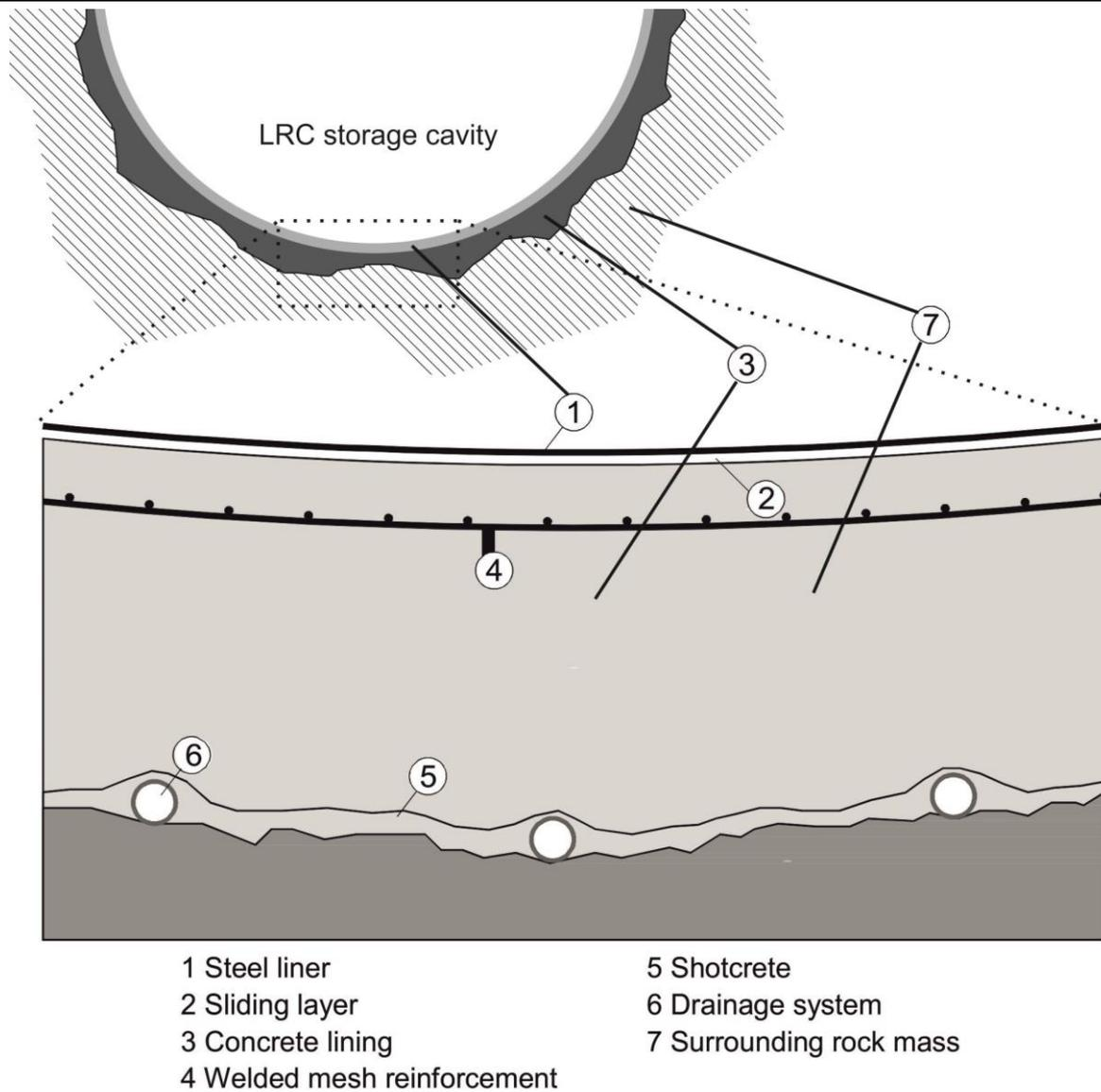
Figure 5-4: Schematic of lined rock cavern wall, after [12] modified by KBB
